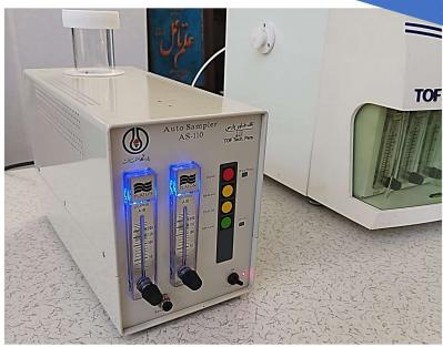
The TOF Tech Gas Auto-sampler (GAS-110) automates the sampling of gaseous samples from cylinders, ambient air, or reservoirs for analysis on an Ion Mobility Spectrometer (IMS) or other sensors. This stand-alone device mixes a fixed volume of the sample with a carrier gas that enters the detector, ensuring precision. The mixing ratio is customizable based on the application, sample concentration, and detector sensitivity.
